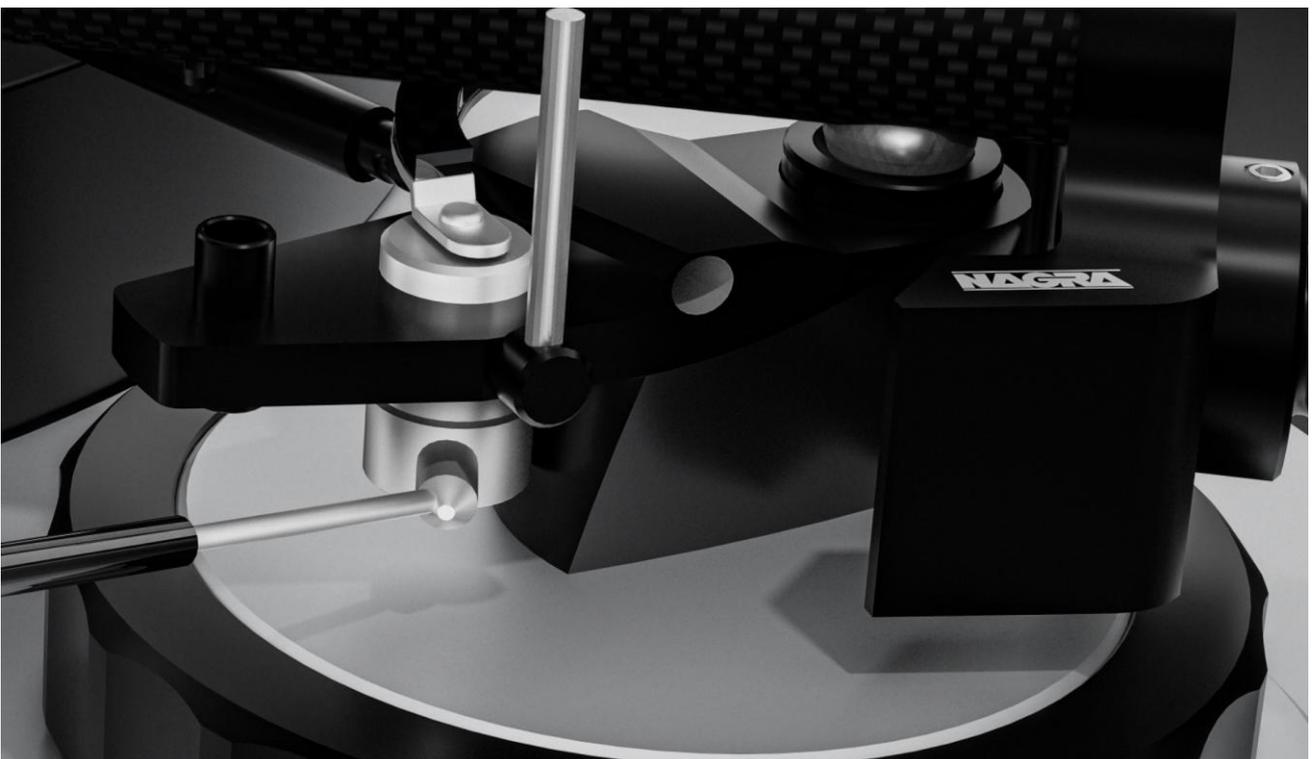
The tonearm's bearing is a simple, extremely precise, CNC machined, hardened steel cone captured in a resonance isolating, silicone damped, ultra high density polyethylene receiving cup. The tonearm's traditional counterweight is supplemented by a low hung, saddle shaped weight providing stability while minimising the tonearm's effective mass.
